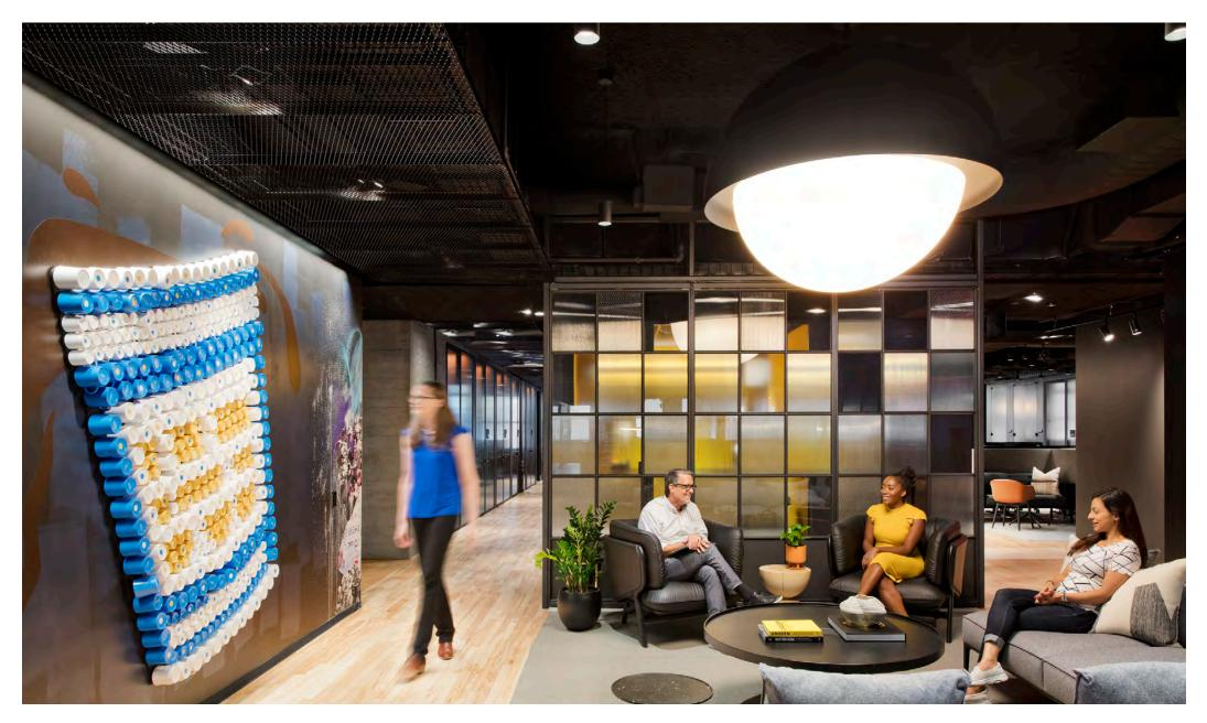
SAS developed the ceiling design intent in close collaboration with Gensler, detailing an expanded metal mesh that provided a surface open area greater than 70% thereby allowing the sprinklers and lights to be positioned above the ceiling membrane thus ensuring a crisp and clean finish.
