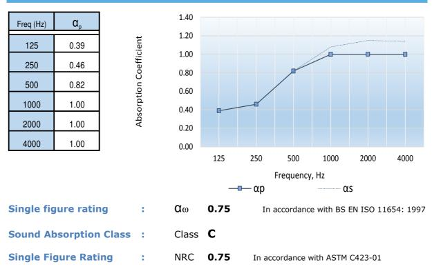
The measurement methodology and associated analysis results in absorption coefficients greater than unity. This is due to diffraction at the edge of the sample and is considered within the measurement standard by specifying the sample dimensions and perimeter detailing.
