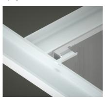
This is a hook-over bracket supplied fixed to the upstand of the panel. Access is obtained by pushing up the opposite end of the panel and sliding back. This reveals the flange which can then be lowered to a vertical position (lift & tilt).
