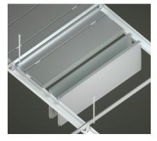
This integral feature allows tiles to be hung vertically from C-Profiles which provides unobstructed ceiling void access. Complete panel runs can be hung together during maintenance without causing damage to the tile. **Flying Arm**
