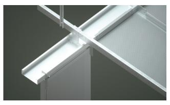
Similar to the flying arm, a hook plate is fixed to the tile edge (supplied loose for on-site fixing by installer). The tile can be completely lifted out of the grid and hooked back over the C-Profile, safely off the ground.
