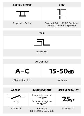
\*Note This includes the entire system and full associated components (suspension, tile, acoustic pad and associated fixings.)
