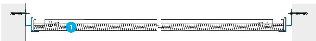
Suspended between walls using perimeter trims.
