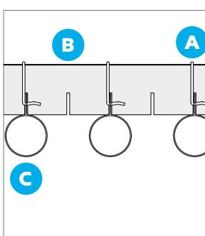
**1** Lightweight installations refer to the ceiling tile and acoustic fleece or pad only. **2** Where the ceiling is expected to support services or upgraded acoustic inlays such as plasterboard or a steel backing plate the loaded installation and the supporting grid should be to the minimum dims shown. Suspension centres should always be considered when applying additional loads. All information from pages 246 - 255 is for guide use only.
