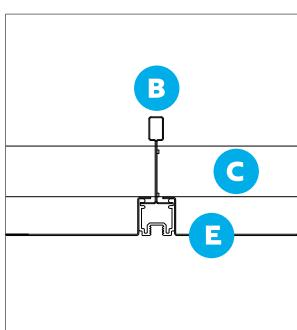
**1** Lightweight installations refer to the ceiling tile and acoustic fleece or pad only. **2** Where the ceiling is expected to support services or upgraded acoustic inlays such as plasterboard or a steel backing plate the loaded installation and the supporting grid should be to a maximum of 3'4" apart for SAS130. Suspension centres should always be considered when applying additional loads. All information from pages 246 - 255 is for guide use only.
