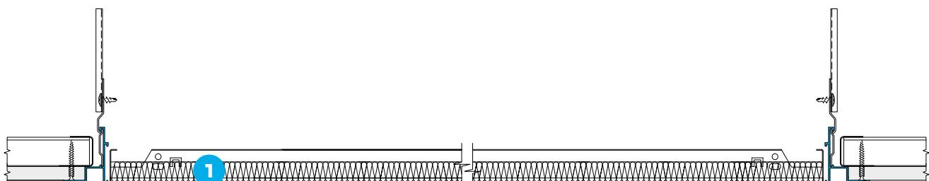
Suspended within plasterboard ceiling.
