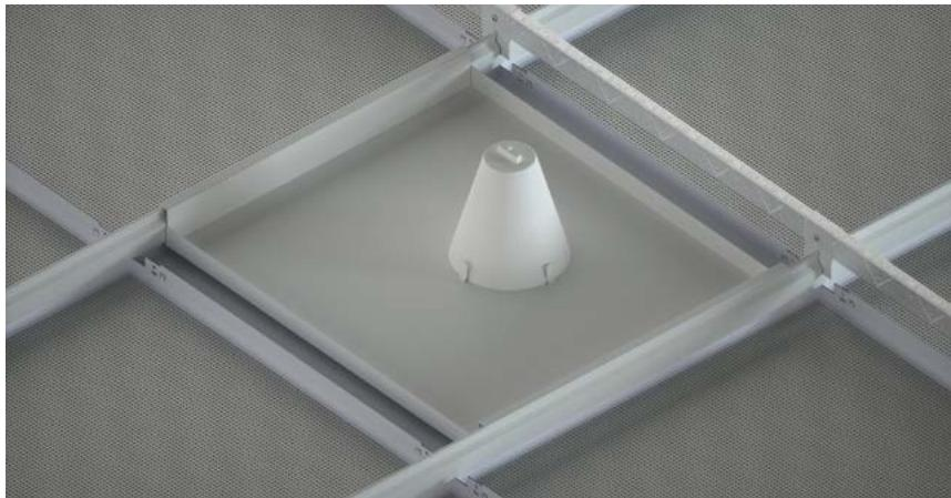
Other services can be integrated with SAS150. Modular lighting can be supported directly from the soffit. Where maximum point loads are exceeded (5lbs) the service must be supported independently or from the grid.
