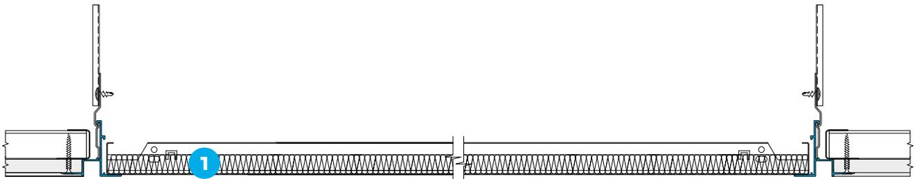
Suspended within plasterboard ceiling.
