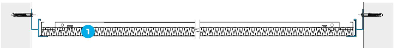
Suspended between walls using perimeter trims.
